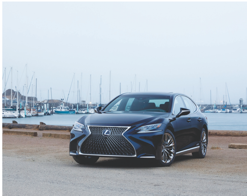
The LS 500h uses a naturally-aspirated 3.5-liter V6 and two electric motor-generators powered by a compact, lightweight lithium-ion battery.
