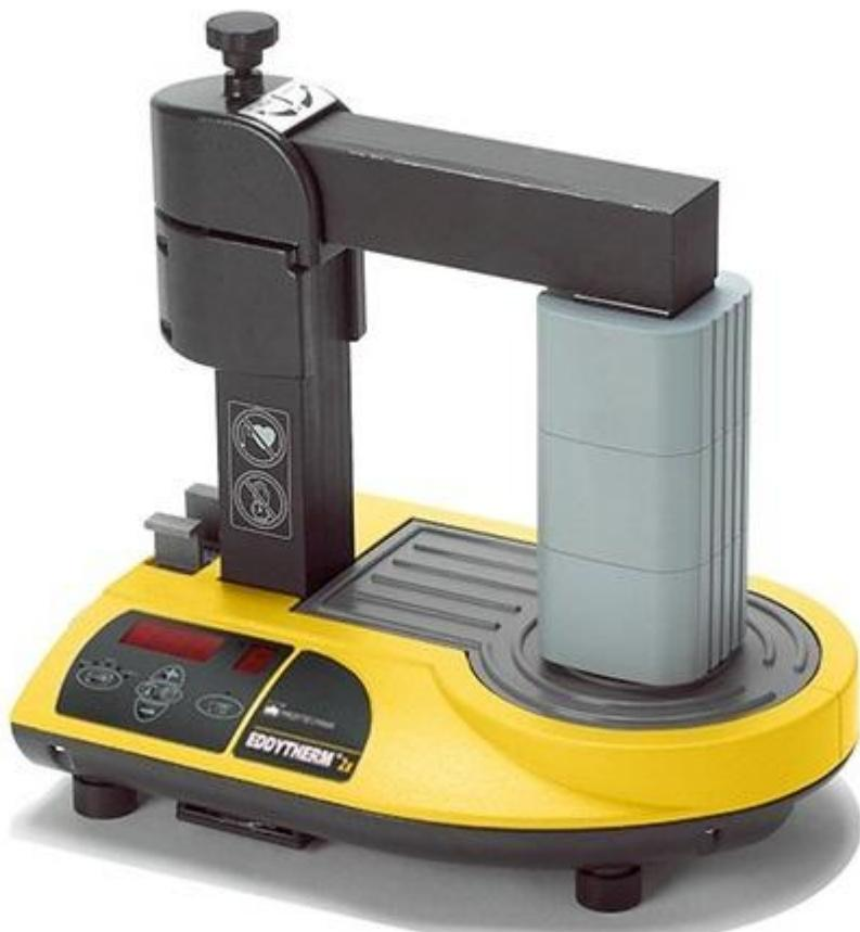
the logical approach to shrink fitting of bearings, gears, couplings,
