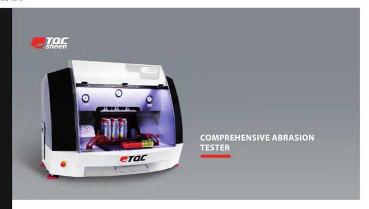
The TQC Sheen Comprehensive Abrasion Tester (CAT) replicates the behaviour of beverage cans during transportation. Failures resulting from scuffing and friction may be very costly for a drinks manufacturer if the result is leaks from a pressurised can wrecking a whole pallet load, or more.
