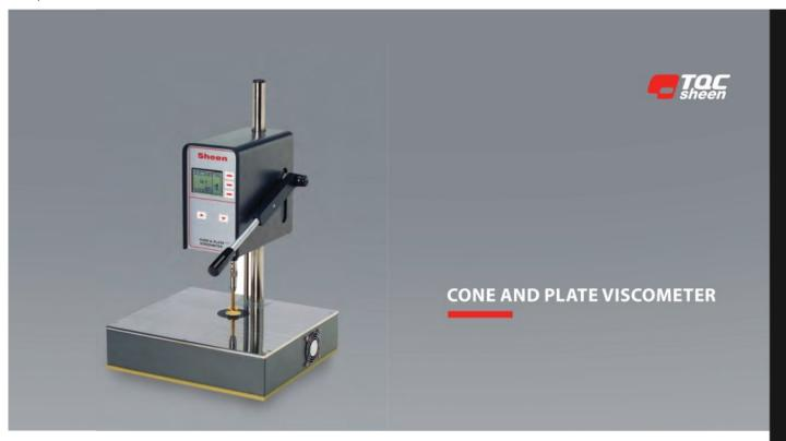
This standard test for dynamic viscosity measurements is now faster and more accurate by use of new high precision microprocessor controls. As non-Newtonian fluids exhibit different viscosities relative to the shear rate applied, the cone and plate viscometer tightly controls it to 10,000S<sup>-1</sup> (B.S. requirements) or to 12,000S<sup>-1</sup> (ASTM). These are generally accepted to be representative of paint application via a roller or brush and so reflect real world' application.
