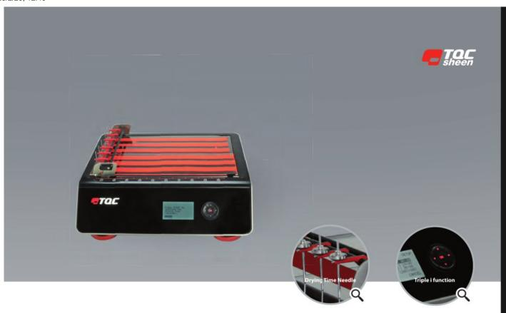
Time Recorder is suitable for fast drying waterborne coatings as well as very slow drying paints.
