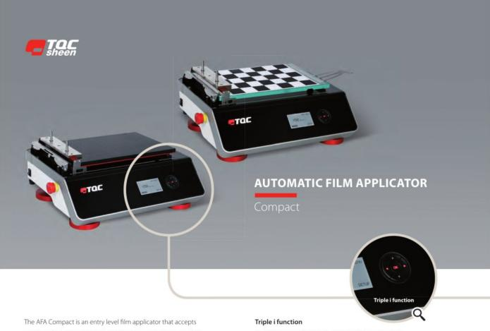
The AFA Compact is an entry level film applicator that accepts charts up to A4 size. Application speed can be set from 1 to 150 mm/s. The Compact is suitable for both wire bar applicators and block applicators. Operating is easy through the standard TQC Sheen operating interface. The AFA Compact is available with a glass bed or a perforated vacuum bed.
