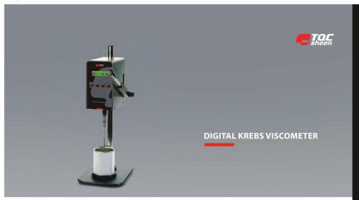
Based on the popular traditional KREBS method, using a weightdriven rotating paddle to sense the paint viscosity at a constant 200 rpm, this modern digital instrument provides automated motor operation, without weights & pulley, allowing accurate direct reading in KU (Krebs units), mPa-s (cP) or g (gram).
