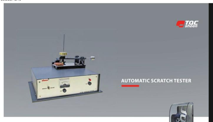
This motorised apparatus is dedicated to coatings hardness evaluation based on scratching resistance method. A test panel is clamped and slowly moved whilst a stylus or alternative tool scratches the surface. Depending on test procedures, specified or variable loads can be applied to obtain different degrees of failure, from trace to destruction. A voltmeter indicates the contact of the tool with the metallic sample substrate.
