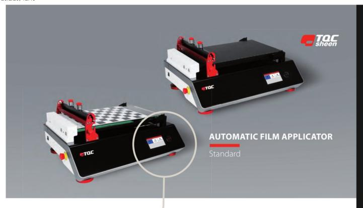
The TQC Sheen AFA Standard provides a reliable basis to apply coating films to test charts, panels or foils in a uniform and reproducible way in order to eliminate variations caused by human factors. Variations in speed, pressure and direction of draw down cause irregularities. Other factors that may influence the result are the shear rate and the weight of the applicator.
