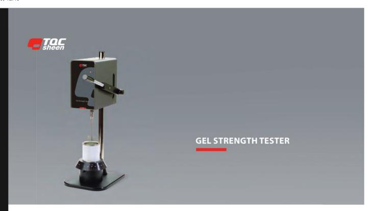
This instrument is especially suited to assess the yield strength and consistency of thick paints and other materials such as gels and putties etc.. A 250 ml can containing the sample is magnetically fastened onto a turntable, which is loaded with a calibrated spring displaying an engraved scale of 0-450 gm/
