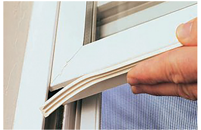
Compressible strips made of foam or another flexible material with adhesive backing works well and are easily installed.
