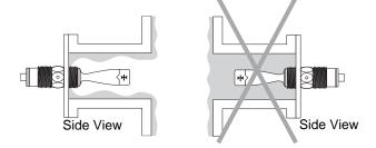
If installing the tuning fork within a pipe, make sure the forks allow the liquid to flow between them and not around them.
