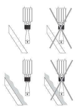
Higher viscosity liquids may build up inside of a flange and cause the NWP to fail wet.
