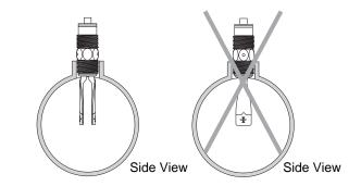
When installing the NWP horizontally, make sure that the forks orientation is vertical and <u>not</u> horizontal.
