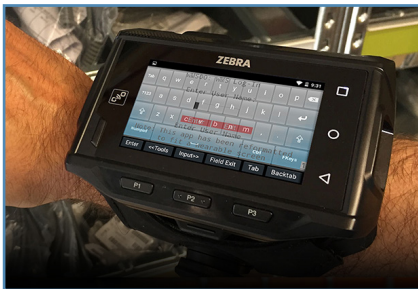
CONFIGURABLE TRANSPARENCY: This configurable feature allows users to see input fields in the background while typing.
