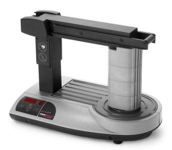
Compact design induction heater for roller bearings and other circular metal work pieces up to 25 inch bore diameter and a cross section of 9-3/4 inch x 9-3/4 inch. With the integrated time and temperature controls, roller bearings can be heated to the prescribed 230°F while other circular metal work pieces can be heated to 750°F. Sliding yoke allows easy loading and unloading.
