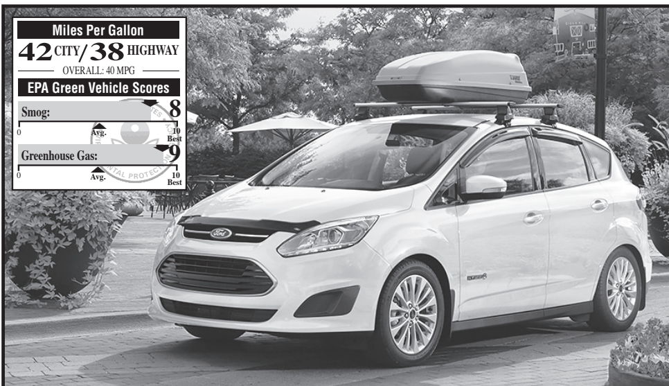
With C-MAX Hybrid, the lithium-ion battery is recharged when the gasoline engine is in operation. Further, regenerative braking can recapture more than 90 percent of the braking energy that would otherwise be lost, using that power to help charge the battery.
