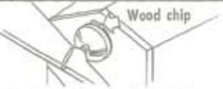
15. Wind the propeller 25-50 turns for power testing, and launch it straight ahead. Gradually increase the winds up to 150-200. If the model stalls under power, cement a small wood chip behind the nose button as shown, to direct the 'pull' downward.
