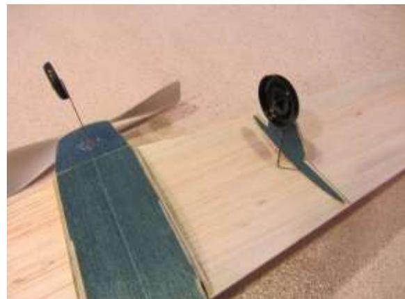
The wheel installation shown is one option. You may have a more desirable setup. The nose wheel is attached directly to the bottom of the nose. This was aided by bending a triangle shape to the wire where it attaches. The main landing gear is attached to the mid-wing rib which incorporates the shape of the gear door. Again, a triangle shape is bent into the wire to aid attachment to the wing.
