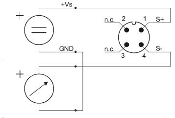
2-conductor, DIN-plug (DRS-...L442)
