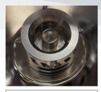
High shear rotor/stator
