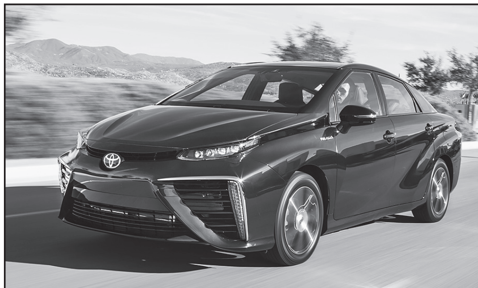
The Mirai hydrogen fuel cell electric vehicle combines hydrogen and oxygen to make electricity onboard, while emitting nothing but water vapor.
