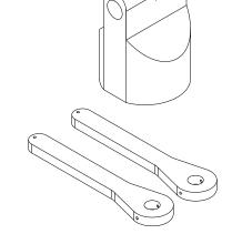
2. Model Supports - Use a .2 mm layer height, 15% fill with no supports.
