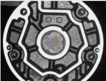
Surface reflectivity difference between the machined aluminum and cast aluminum (direct vs. scattered light)
