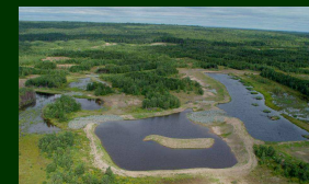
Constructed wetlands provide wildlife habitat, reduce sedimentation of streams and attenuate flashy flows.
