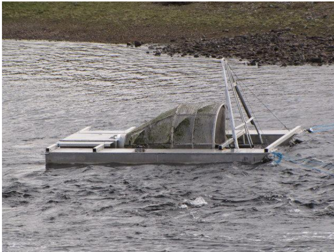
ROTARY FISH TRAP CAPTURES SEAWARD MIGRATING SMOLT
