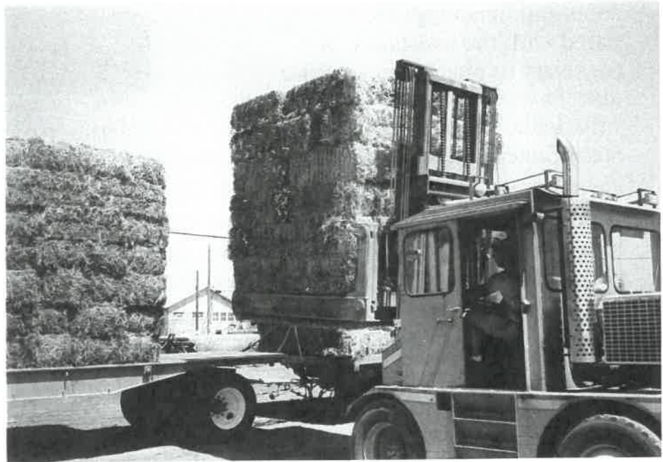
The Roadrunner Squeeze, developed in the late 60's allows one man to pick up a full harrow bed stack of bales and move it quickly and efficiently.
