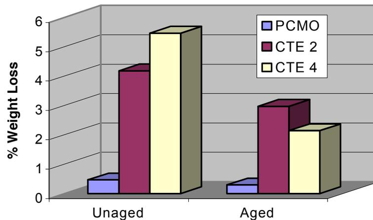
**Figure 1. Abrasion resistance of E-Krete PCMO compared to coal tar emulsion using a modified form of the wet track abrasion test.**
