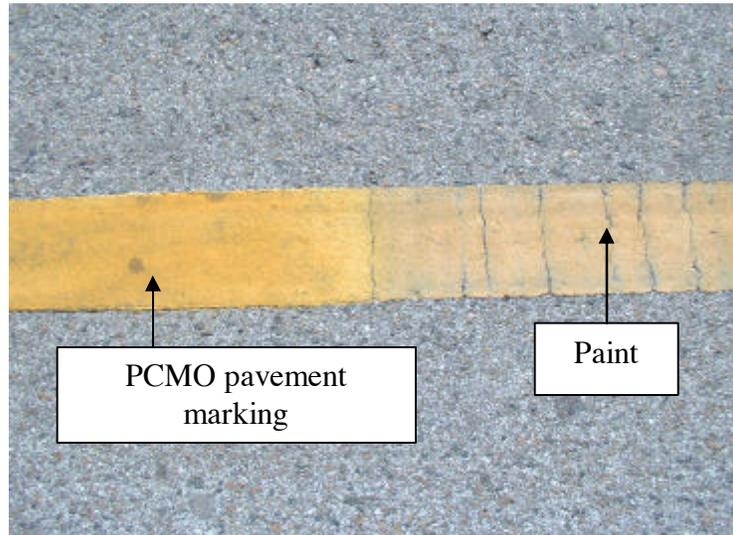
**Figure 6. PCMO pavement marking line at MacDill AFB in October 2012 after 4 full years in service. Note the transverse cracking in the conventional airfield pavement marking paint. The marking paint is approximately 3 years old in this picture.**
