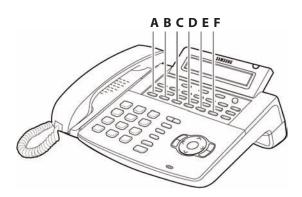
pulse to tone conversion. If your system uses rotary (or pulse) dialing C.O. lines, pressing **D** while entering a speed dial number causes all subsequent digits to be sent as DTMF tones.
