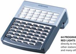
64 PROGRAMMABLE KEYS WITH RED LIGHTS Used to call stations directly, to indicate busy conditions of other stations, for One Touch dialing and many other system features.
