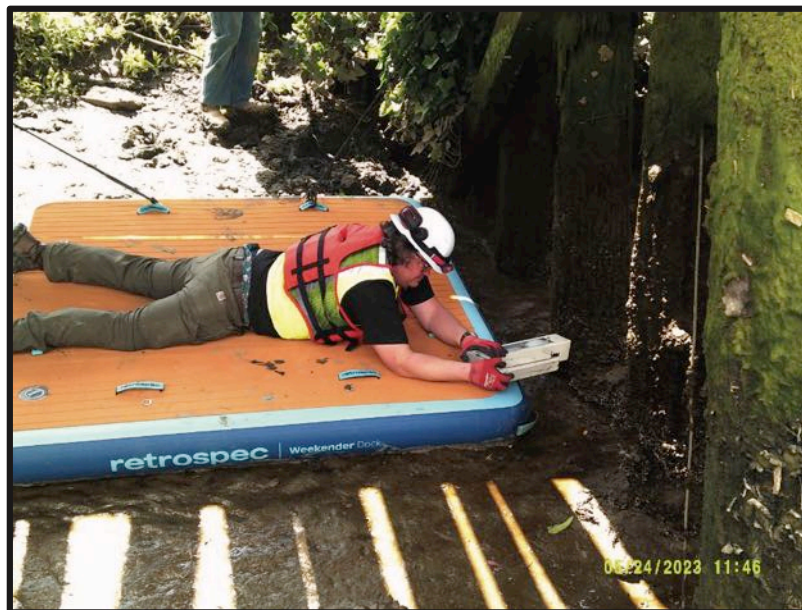
Figure 8. Resistance drilling of a timber pile near mudline at low tide.
