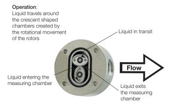
The positive displacement flow technology allows for precise flow measurement of most clean liquids regardless of the media's conductivity. Other liquid properties also have a minimal effect on the performance of this type of meter. Flow profile conditioning is not required, as with alternative flow technology options, making oval gear installations simple to install in tight spaces and at a economical price.
