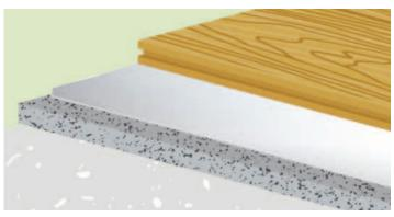
FILM SIDE UP when applying to concrete.
