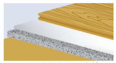
FILM SIDE UP when applying to wood subfloor.
