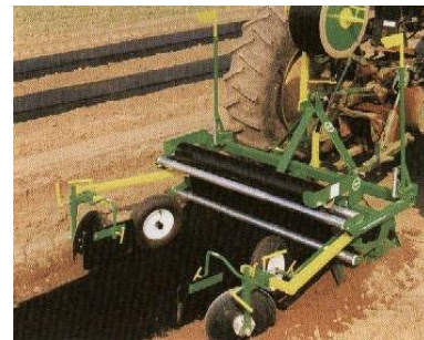
Mulch layer w/drip attachment
