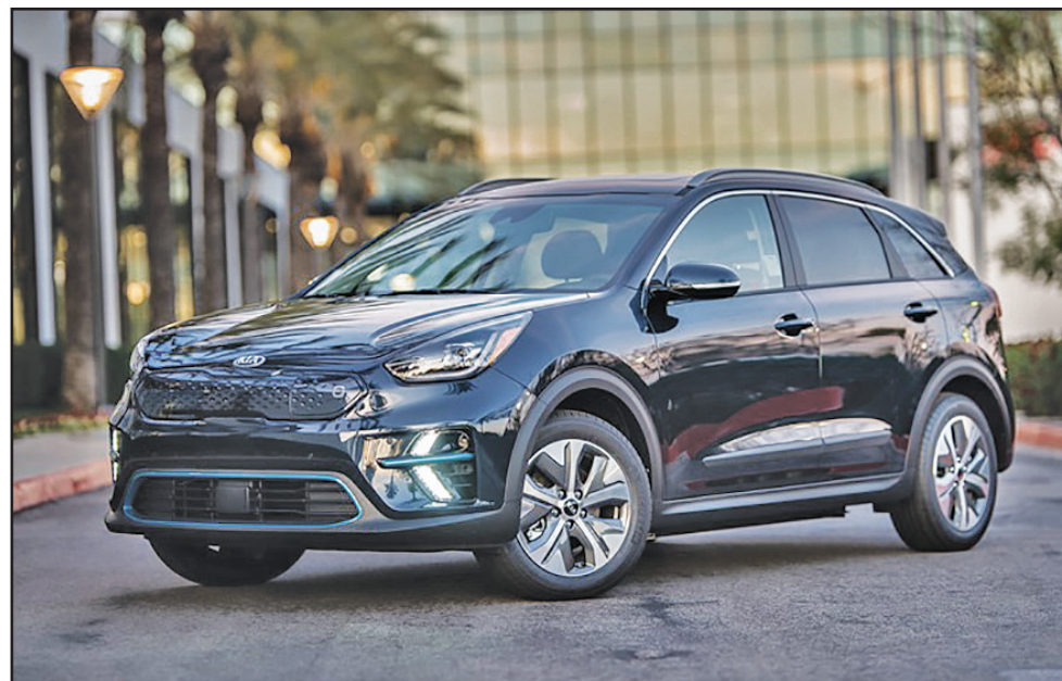
Unique front fascia with closed off grille – no need for an open grille, since there's no internal combustion engine to cool.
