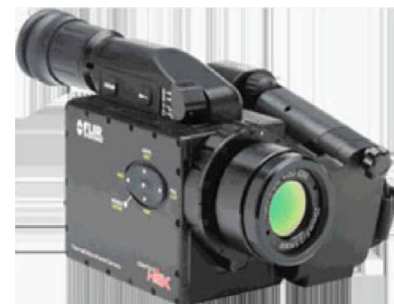
FIGURE 1. Fugitive emissions cannot be seen by the unaided human eye ( www.engineerlive.com ). Specialized cameras can identify and quantify fugitive releases of several different VOCs ( www.irtconsult.com ).
