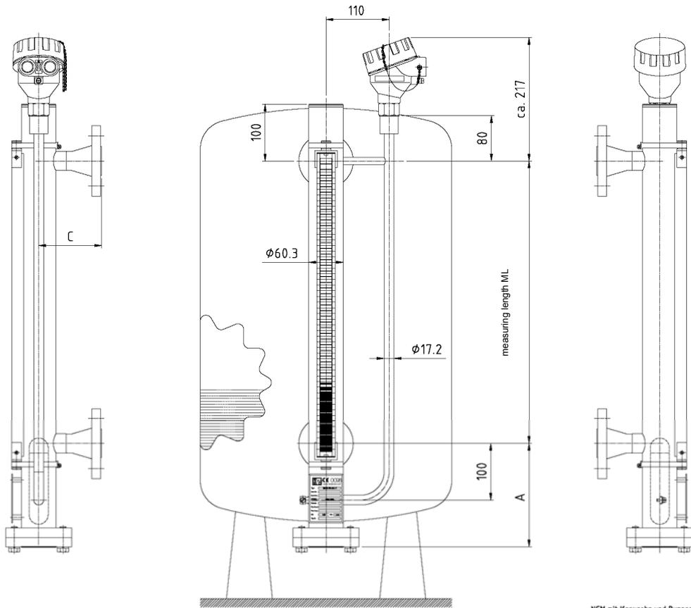
**NGM assembled in a bypass tube with roller/ball display (redundant measurement) option K**
