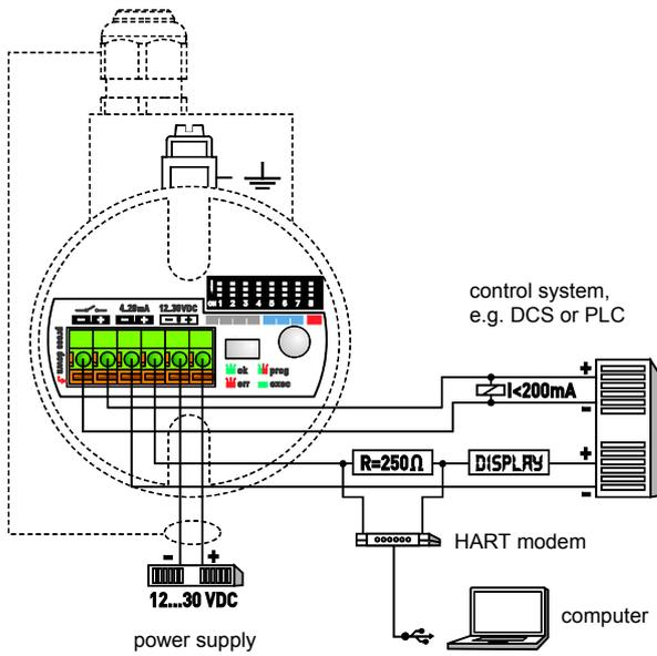
Figure 8: wiring
