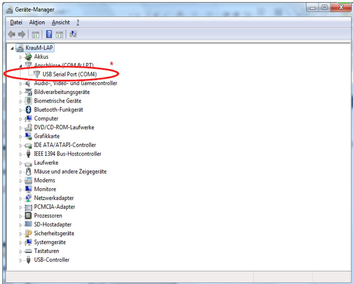
\* In this case COM port 4 has been assigned to the HART modem
