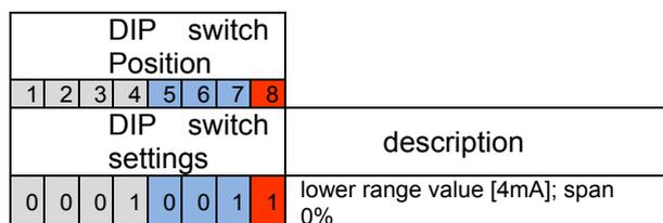
**Figure 12: lower range value [4mA]; span 0%**
