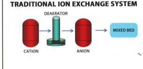
Cation and anion vessels remove ions from the water. Deareator removes carbon dioxide. Mixed bed final polishes the water and removes any remaining ions from the water.
