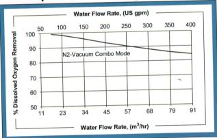
Curves represent nominal values, generated using water at 20°C. O<sub>2</sub> Removal: 14x28 inch, X40 membrane, N2-vacuum combo mode, vacuum: 75 mm Hg, N2 Sweep 0.5 scfm.
