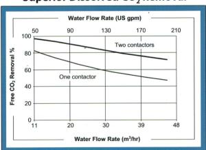
Curves represent nominal values, generated using water at 20°C. CO<sub>2</sub> Removal: 14x28 inch, X50 membrane, Air vacuum combo mode, vacuum: 150mm Hg, air sweep 8 scfm.
