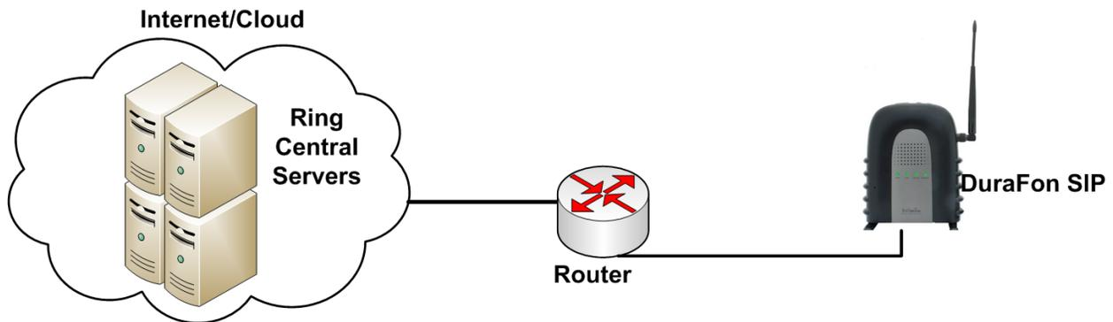
*Note: In order for this setup to work the Gateway (router at the demark), must be properly configured for the Ringcentral cloud services to establish a connection and operate properly. Please consult with the networking equipment vendor in order to ensure the networking equipment is properly configured.*
