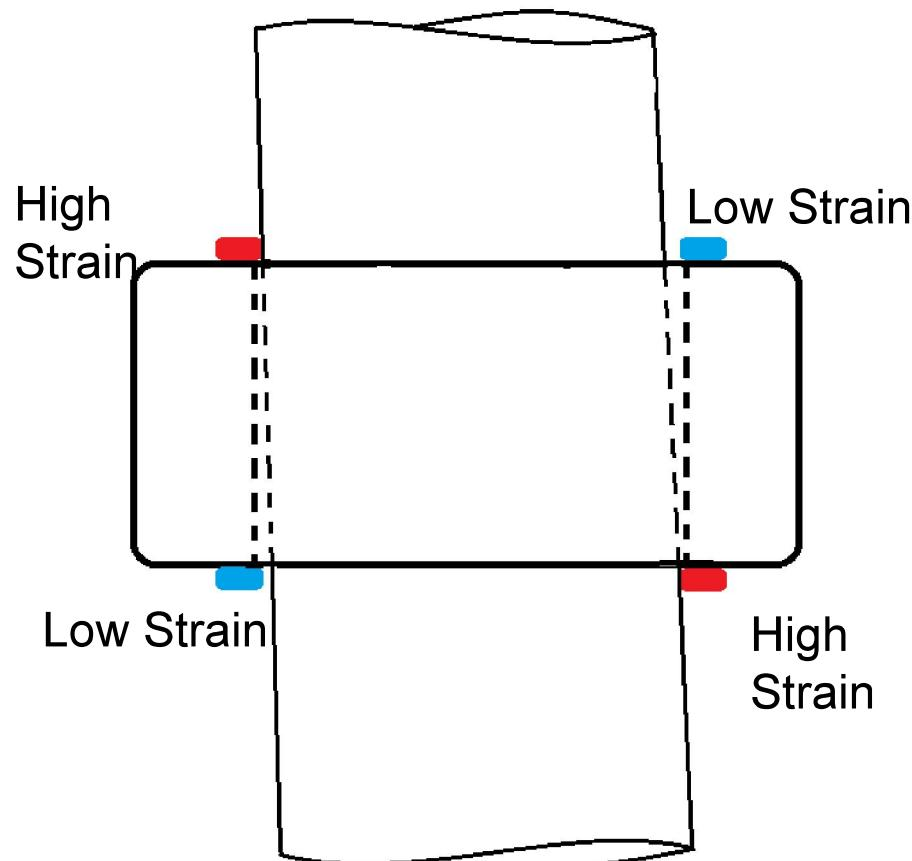
Note: Strains should be similar on both faces of the bearing during slow roll
