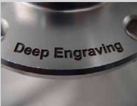
Metals: engraving & deep engraving on metal
