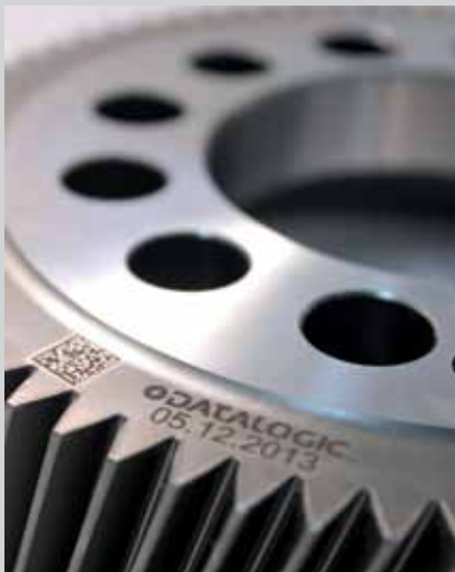
High contrast marking on metal
