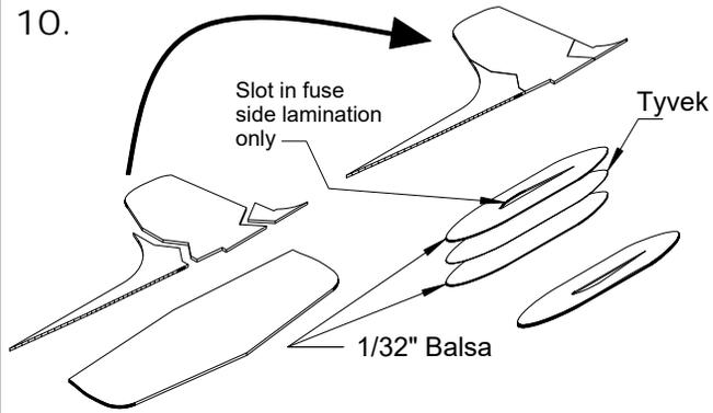
Cut out the tail surfaces from 1/16" balsa. Sand both surfaces to a symmetrical cross section (not shown in these illustrations). Also cut out the two tip tank parts from 1/32" balsa and Tyvek. Assemble the tip tanks and then sand the edges round.
