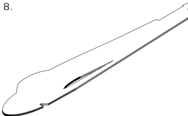
Once the glue dries in the fuselage lamination lay up, cut out the fuselage.
