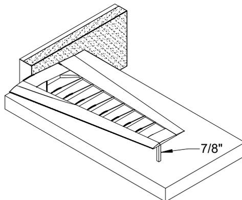
Block each wing panel up 7/8" at the tip with the root flush with the building surface. Sand the root of each panel so the wing panels can be joined in the middle with 7/8" dihedral under each wing tip.
