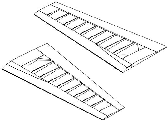
When all of the glue is dry, remove the two wing panels from the plan. Sand the wing panels to the airfoil shown in the wing root cross section shown on the plan. Taper the wing thickness toward the tips.
