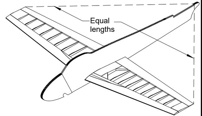
Slide the wing into the fuselage slot. Make sure the wing is square to the fuselage and glue it in place.
