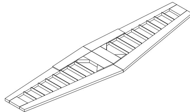
Cut some firm 1/32" balsa into several 1/4" wide strips. Using the 1/4" wide strips, cut and glue individual lengths at each rib location.
