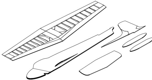
Cover the wing, fuselage, fin, and tip tanks (not shown in these illustrations).
