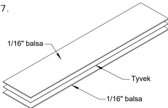
Cut two pieces of 1/16" balsa to slightly larger than the length and width of the fuselage. Also cut a piece of Tyvek to the same size. A good source of Tyvek is a U.S. Priority Mail envelope. Glue the laminations together with a glue like Titebond or a cellulose based glue like Sigment.
