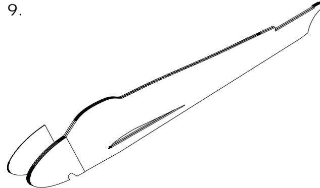
Sand the fuselage to form a cross section similar to the one shown on the plan (not shown in these illustrations). Glue the 1/64" plywood nose doublers to each side of the fuselage. Sand the doubler edges when the glue is dry.
