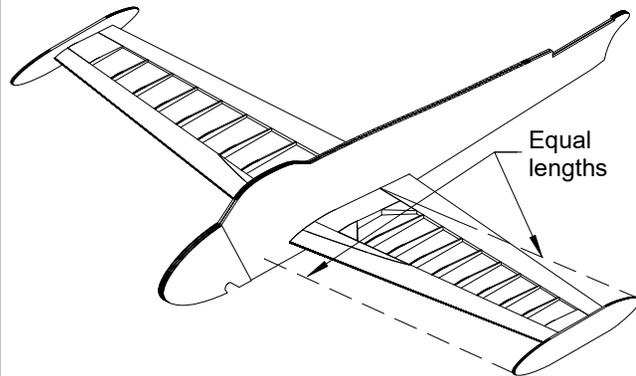
Glue the tip tanks to the wing tips. Use the plan as a locating reference. Measure the distance from each tank tip to the fuselage. Make sure the distances are equal.
