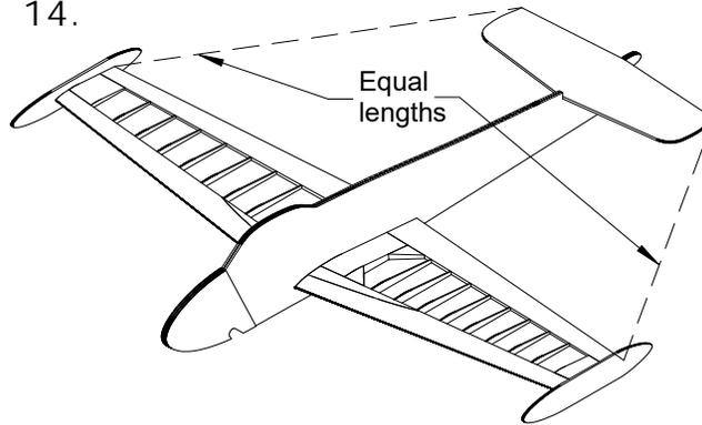
Glue the stab to the fuselage. Make sure the distance from each stab tip to its corresponding wing tip is the same distance.
