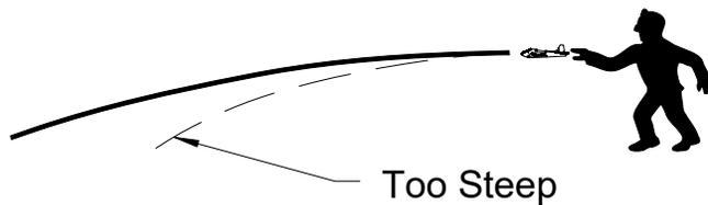
Hand glide the model. If it tends to glide too steeply or dive, add a little up elevator. This was done with the prototype rather than sanding down the Budkickers. The goal was to keep a nice margin of positive stability while still not looping during the launch phase.
