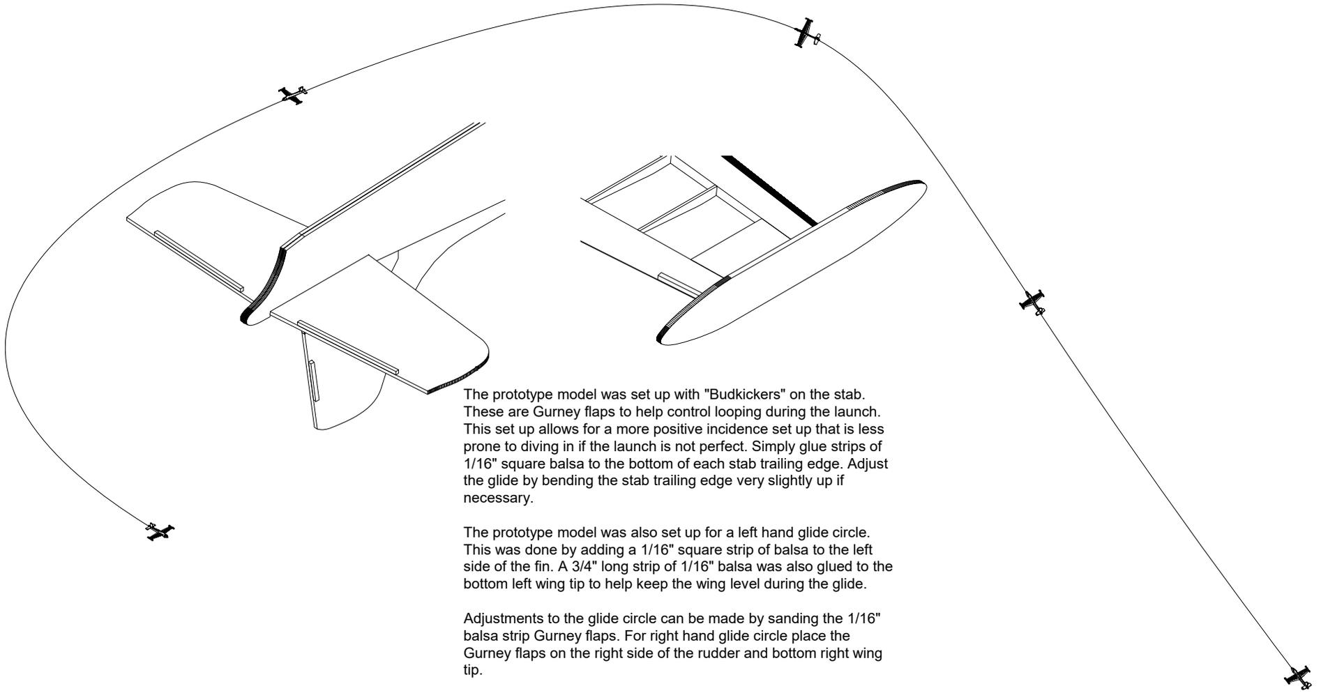
The prototype model was set up with "Budkickers" on the stab. These are Gurney flaps to help control looping during the launch. This set up allows for a more positive incidence set up that is less prone to diving in if the launch is not perfect. Simply glue strips of 1/16" square balsa to the bottom of each stab trailing edge. Adjust the glide by bending the stab trailing edge very slightly up if necessary.
