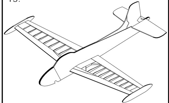
Glue the fin to the fuselage and stab.
