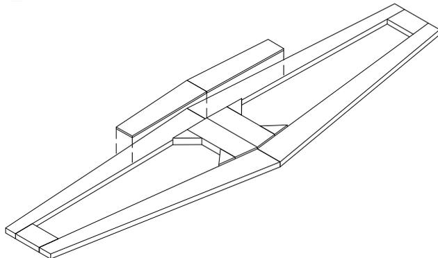
Cut the wing outline parts from 3/16" and 1/4" balsa. Glue the outline parts together using the plan. DO NOT glue the center section joint. Also glue the 1/16" balsa laminations to the LE.
