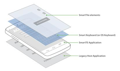
SmartTiles: A Layered Approach — Because SmartTiles are located 'above' the application layer, this allows you to position components anywhere on the screen without interfering with text fields, labels, keyboards or other critical application elements.
