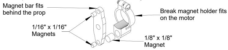
While not necessary, it has been found that using a prop adapter on the motor can make the use of the magnetic brake easier to set up. It also makes the overall installation of the prop much easier. The prop adapter being used is made from a DuBro threaded pushrod coupler for 1/16" diameter pushrods.
