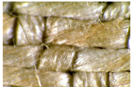
Figure 5. The Information is Encoded into the Location of the Discoloration on the Fibers.
