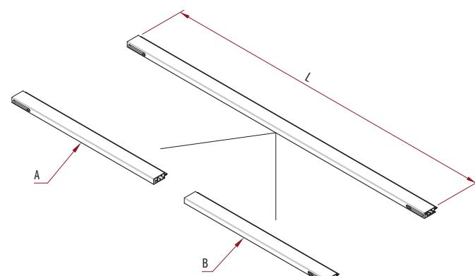
Take the cut pieces and insert them into the ceiling and the base of the wall unit take care to always position the lip in the part inside the cabinet.
