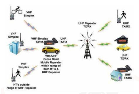
In order for repeaters to receive a signal and transmit a signal simultaneously, they have to "listen" and "talk" on two different frequencies. The frequency that you will HEAR a repeater on is regarded as the repeater's "home" or "transmit" frequency. This is where you will find the repeater in repeater listings and directories. This "home" or "transmit" frequency will be the frequency that the repeater transmits on, and you will LISTEN to it on.
