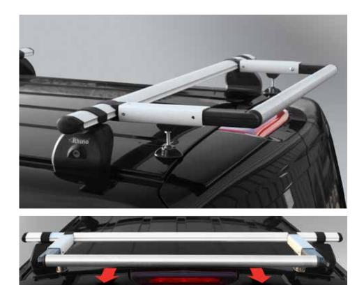
The KammBar<sup>®</sup> rear roller retains the same virtues as the KammBar<sup>®</sup> of both strength and modern styling combined, with features such as adjustable supports to allow for the optimum position of the stainless steel roller.
