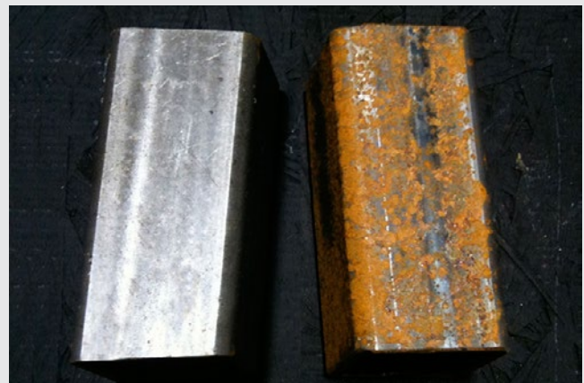
With Protection Without Protection Humidity and Salt-Spray Testing ASTM D-1748
