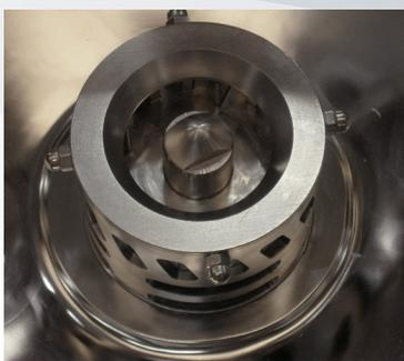
High shear rotor/stator
