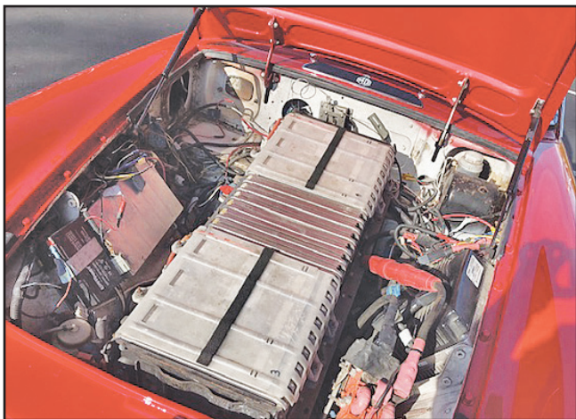
Vijay obtained two 2013 Nissan Leaf batteries and placed parts of them in the rear compartment and under the hood.
