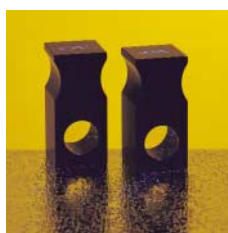
For regular conformance testing the colorimeters are also supplied with a certified glass filter of specified colour value.
