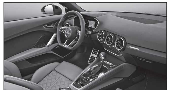
The virtual cockpit combines the functions of a central MMI® system with a traditional instrument cluster.
