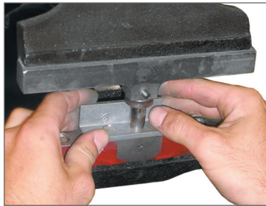
Bench vise used vertically as a press.
