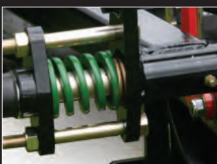
Wing unit spring to minimise collision damage
