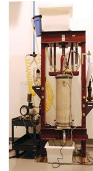
Acoustic Emission Testing of Ultralite Composite Pressure Vessels at manufacturer's facility in ROCK HILL, SC
