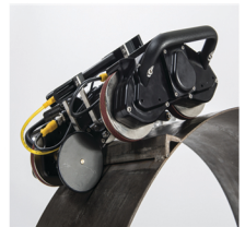
Ultrasonic Thickness Testing being conducted via Remote Magnetic Crawler.
