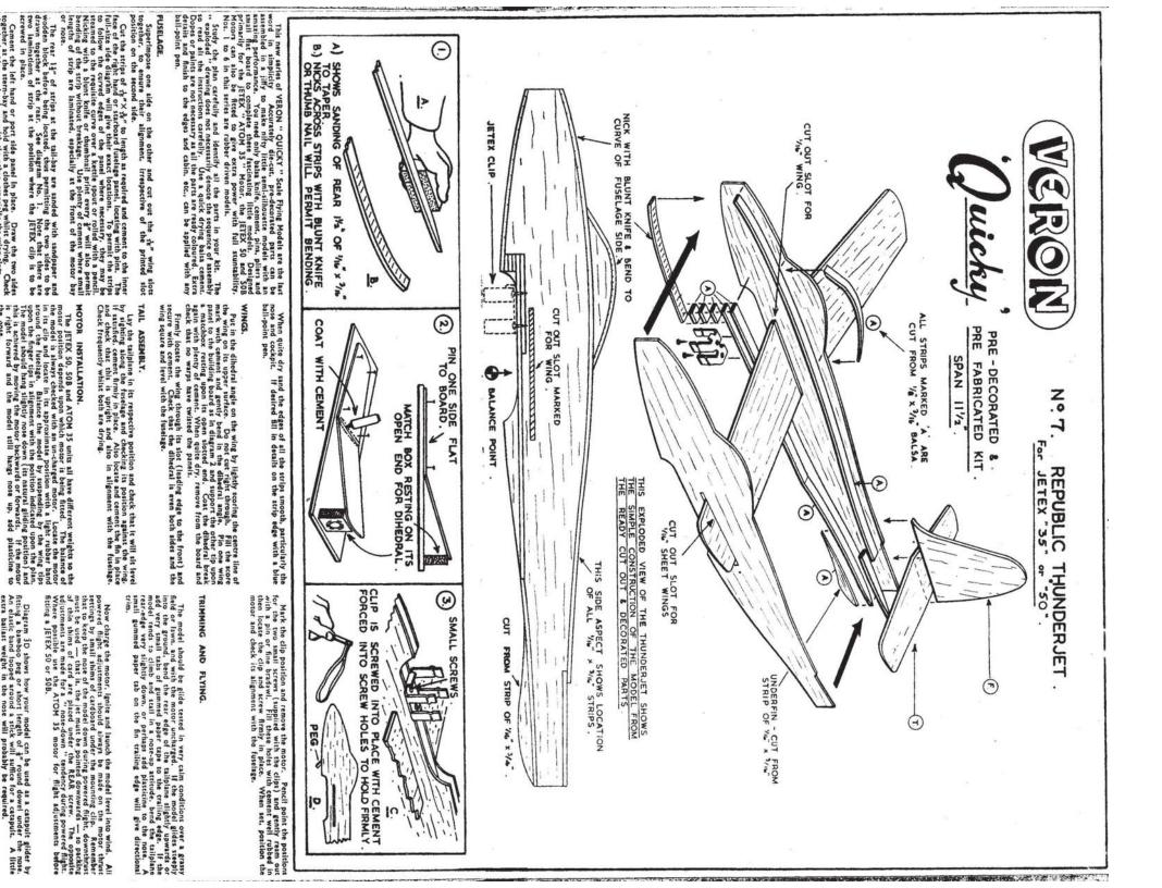
MODEL AIRCRAFT ( B'MOUTH) LTD. NORWOOD PLACE Cement the left hand or port side panel in place. Draw the two sides together at the stern-bay and hold with a clothes pege whilst dring. Check that both sides are level one with the other, especially the wing slots.
