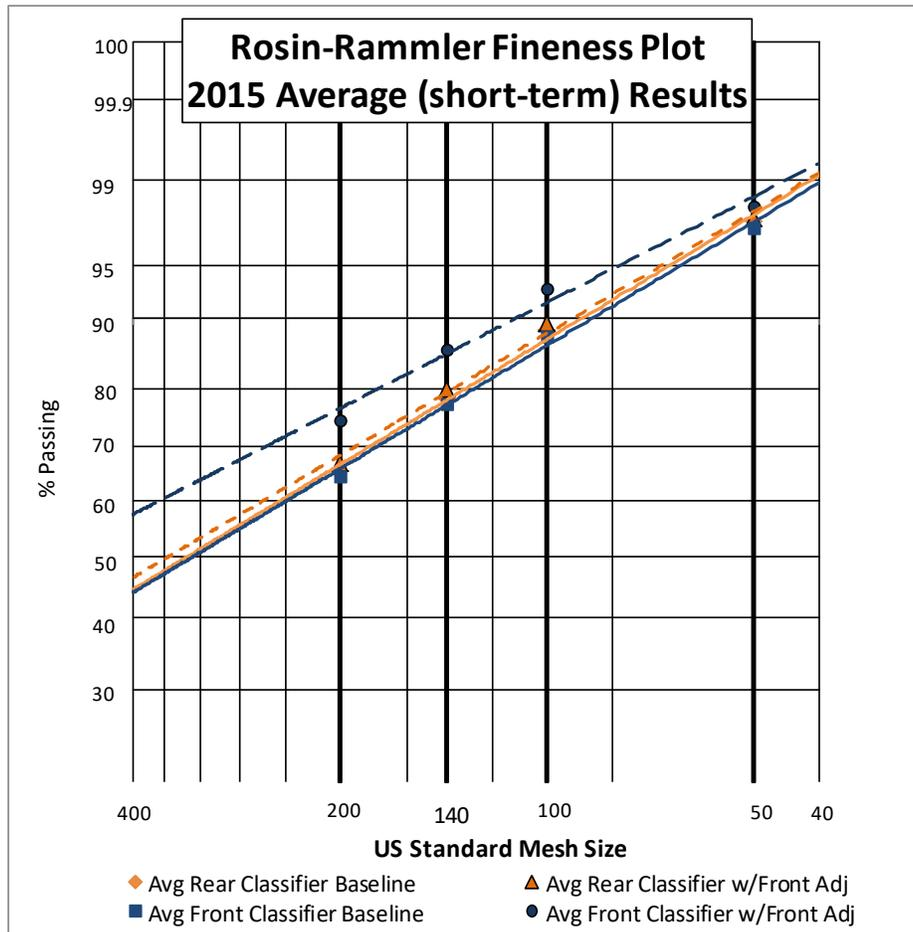
**Figure 4: Average 2015 fineness test results before and after front wall classifier and orifice adjustments.**
