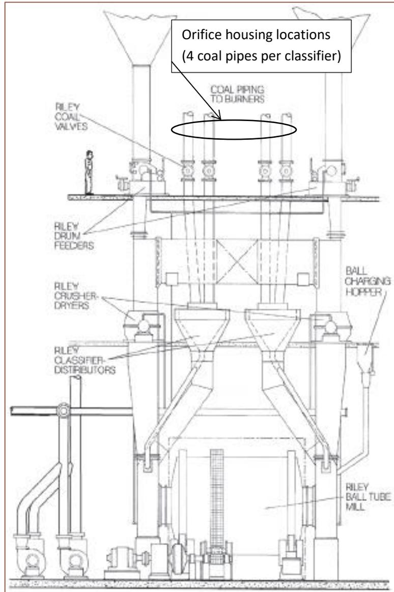
Figure 1: Typical mill layout. (Riley Power)
