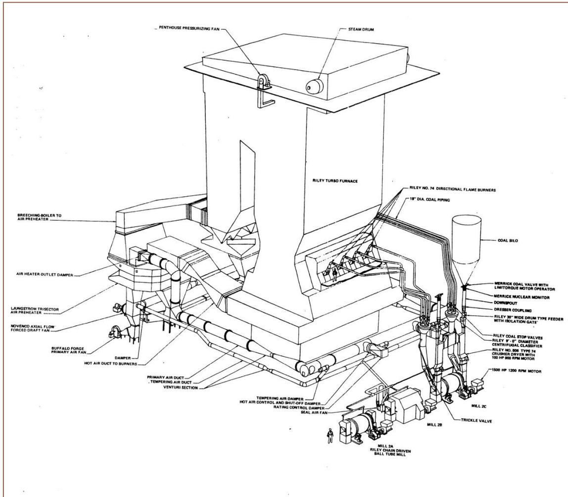
Figure 2: Unit layout. (Riley Power)
