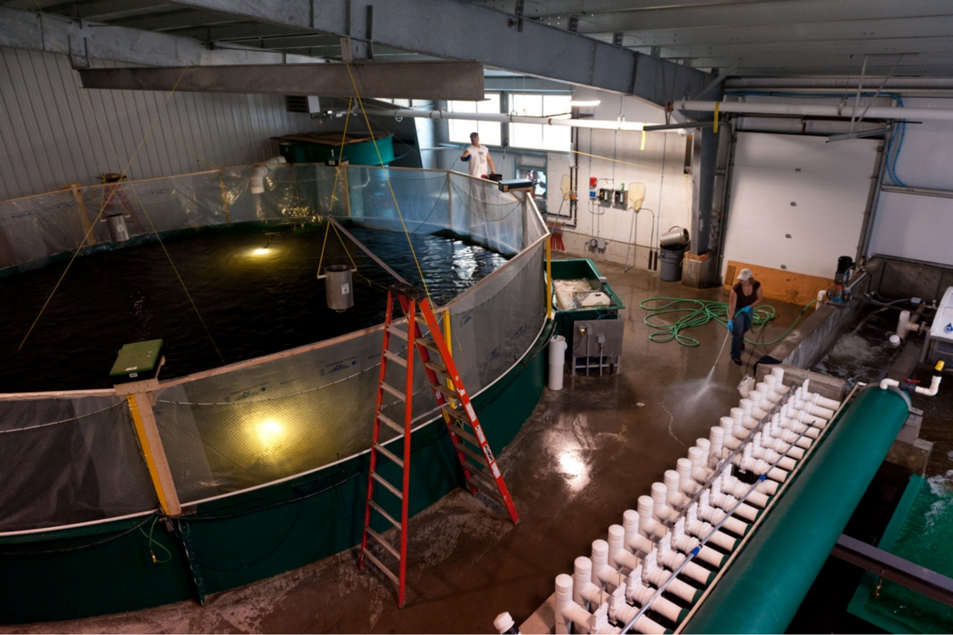
Quarantine Facility 1 tank 250 m 3 & 11m diameter
