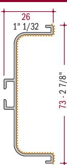
"GOLA" HORIZONTAL ALUMINUM SPACER CHANNEL PROFILE FOR BASE CABINET
