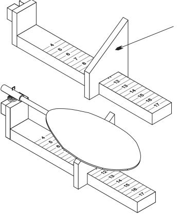
MOVE SLIDER TO SET THE DESIRED PITCH. MOVING THE SLIDER OUT INCREASES THE PITCH VALUE.
