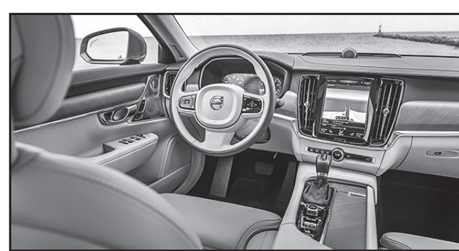
The interior makes use of the Sensus Connect touchscreen that debuted in the XC90, providing a clutter-free interior with minimal dashboard buttons.
